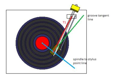
The angle between green groove tangent line and T1 tonearm stylus-pivot line is more than (zero) 0 degrees because groove tangent line does not pass through the tonearm pivot. So there will be skating force, even it does not have an overhang, but because of this lack of overhang there will be a much less side-force.
