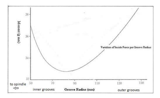
It is a graph showing one tonearm example of a typical variation of side-force per groove radius in overhung tonearms.
