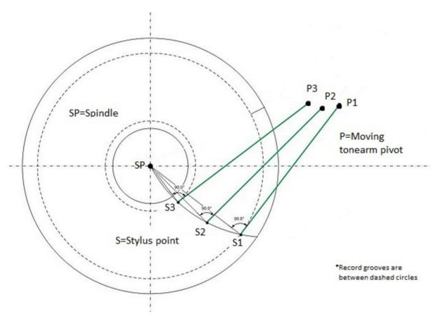
As you can easily see, at every tonearm position, groove tangent line is passing through tonearm pivot, and because pivot is not fixed but moves accordingly, the angle between groove tangent line and stylus-pivot line remains 0 (zero) degrees.
