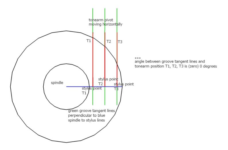
As you see, because tonearm pivot is not fixed and moving accordingly, at every position of the tonearm, groove tangent lines always passing through the tonearm pivot and angle between groove tangent line and tonearm stylus-pivot line is 0 (zero) degrees.
